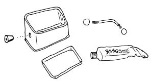
At a hardware store, get a 5/32" brass rod. (They come in foot-long pieces.) Get two brass balls of the sort you screw onto lamps to hold the lampshade on, the ones that are threaded 8-32. Get a rubber cork, tapered, about a half inch in the middle. It should have a hole running its length to hold the brass rod tightly.
